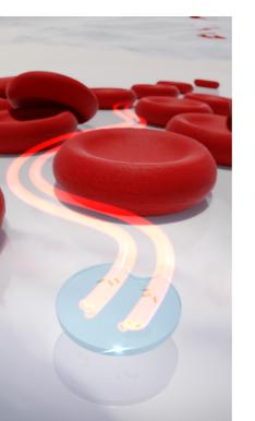
The highly steerable microdrones are significantly smaller than red blood cells (above). Whereas the mode of generating thrust is entirely different, the combined effect of the different nanomotors is conceptually similar to that of the rotors on a guadcopter drone (left).
