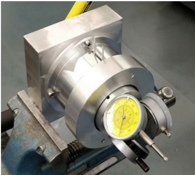
Fig. 1: The clutch test bench for gaining initial experience with the relaxation stroke and the friction force.
