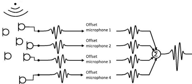
Beamforming principle for acoustic waves<sup>3</sup>
