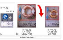
Not only can the PISC prototype replace a larger capacitor. The size and mass of necessary complemental chokes is even more stronaly reduced (above). Due to the extent of filtering components in a typical power supply (left, red boxes), the savings potential is significant.
