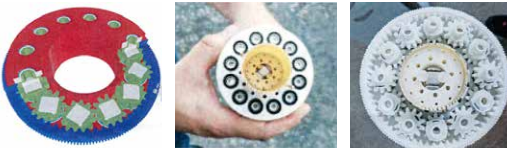
Fig. 1 - 3: CAD model and 3D-printed, working demonstrator of the "Halbach Gearbox".
